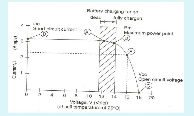
Source: Mark Hankins (2010) Figure 5. Typical Characteristics of Solar PV Modules
