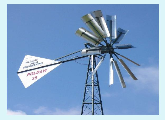
Drag Type wind Turbine for Water Pumping
